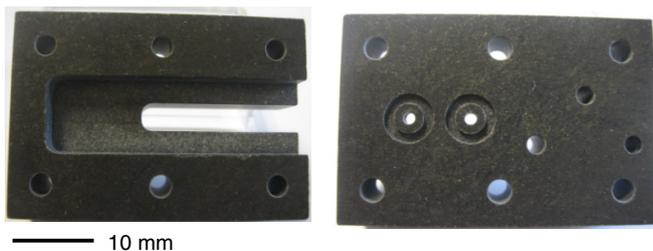
Figure 6. Machined package parts.
