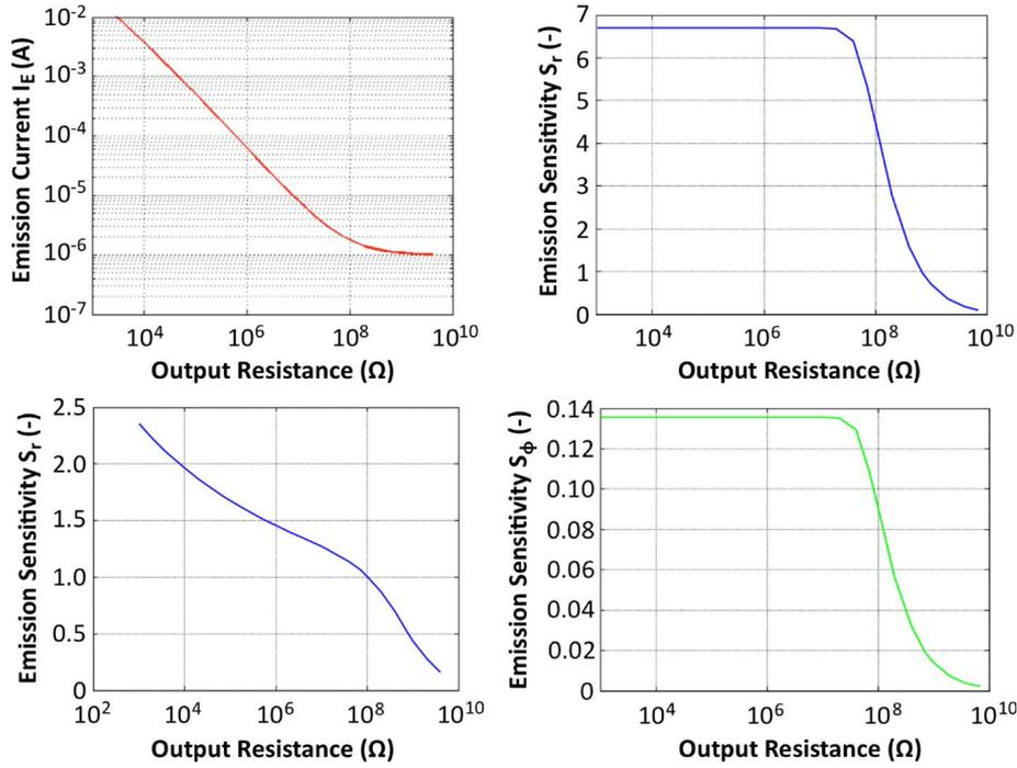
Fig. 5. (Top left) Emission current, (top right)  $S_r$  for  $\Delta r = 5$  nm, (bottom left)  $S_r$  for  $\Delta r = 1.5$  nm, and (bottom right)  $S_\phi$  versus output resistance for an FET/FE unit with  $r_o = 30$  nm,  $\phi = 4.5$  eV,  $\Delta\phi = 0.2$  eV, and  $I_{DSS} = 1$   $\mu$ A.
