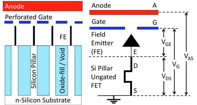
Fig. 3. (Left) Device structure. (Right) Equivalent circuit. Each FE is formed on top of a different silicon column (i.e., ungated FET). The bias voltage  $V_{GS} = V_G$  is divided between the voltage across the FE (i.e.,  $V_{GE}$ ) and the voltage across the FET (i.e.,  $V_{DS}$ ), i.e.,  $V_G = V_{GE} + V_{DS}$ .
