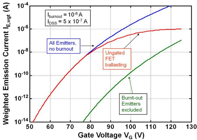
Fig. 8. Weighted  $I$ - $V$  characteristics of an FET/FEA structure, weighted  $I$ - $V$  characteristics of the FEA if no FETs are present and no emitter burnout occurs, and weighted  $I$ - $V$  characteristics of the FEA if no FETs are present and emitter burnout occurs.
