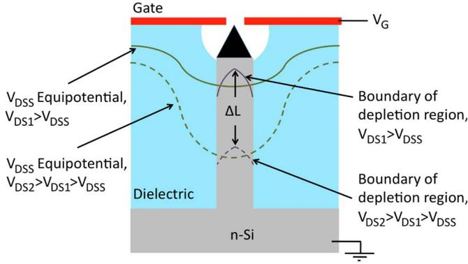
Fig. 4. Schematic diagram depicting the depletion region and equipotential lines for a single FET/FE.
