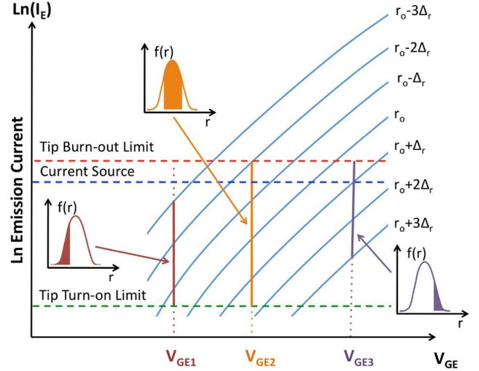
Fig. 1. Semilog plot of the family of  $I$ – $V$  characteristics from a single tip for an FEA that has a tip radii distribution with average radius  $r_o$  and radius variation  $\Delta r$ . For a constant bias voltage, only a small fraction of the tip array emits current.
