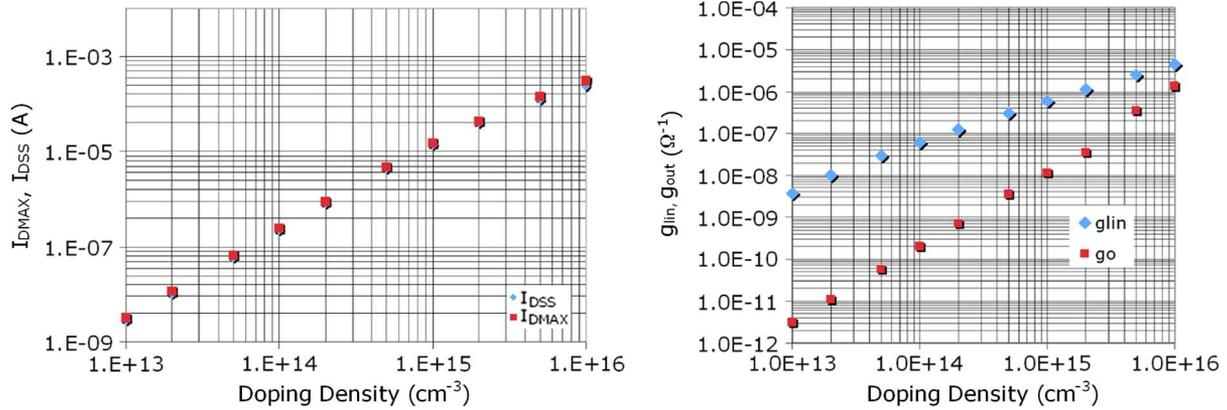
Fig. 6. (Left) Drain-to-source saturation current  $I_{DSS}$  and maximum current at 100 V  $I_{DMAX}$  and (right) linear conductance  $g_{lin}$  and output conductance  $g_{out}$  versus doping concentration for a  $1 \mu\text{m} \times 1 \mu\text{m} \times 100 \mu\text{m}$  ungated Si FET.
