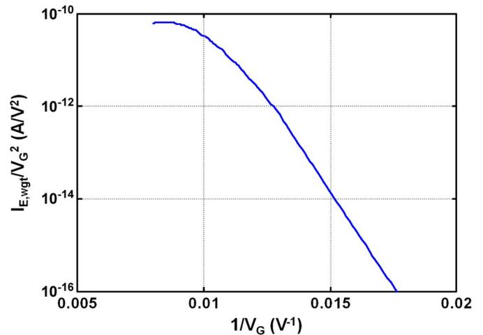
Fig. 9. For a low bias voltage, the weighted  $I$ - $V$  characteristics of an individually ballasted FEA describe a straight line with negative slope in the FN plot. For large bias voltages, the current limitation by the FETs forces the slope of the FN plot to increase until it becomes horizontal. Further increase of the bias voltage will make the slope become positive.
