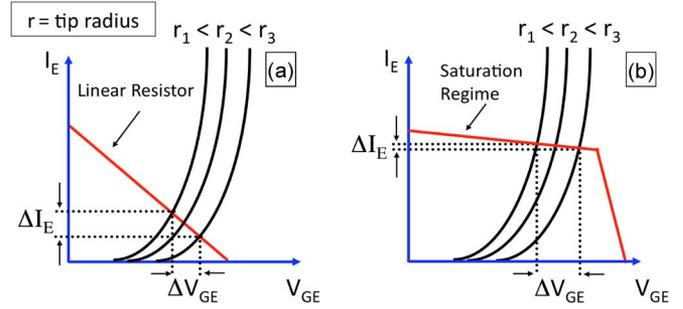
Fig. 2. Negative feedback of an FE using (a) a linear resistor and (b) an ungated FET. In the first case, low emission current variation within the FEA is achieved using a very large linear resistance, which results in low-current emission. If an ungated FET is used instead, both low variation and high-current emission are achieved because the current uniformity depends on the magnitude of the output resistance of the FET, which is to first order independent of its saturation current.
