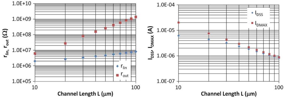
Fig. 7. (Left) Linear resistance  $r_{lin}$  and output resistance  $r_{out}$  and (right) drain-to-source saturation current  $I_{DSS}$  and maximum current at 100 V  $I_{DMAX}$  versus channel length for an ungated FET with  $1 \mu\text{m} \times 1 \mu\text{m}$  cross section and  $2 \times 10^{14} \text{ cm}^{-3}$  doping concentration.
