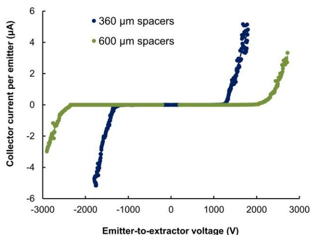
Fig. 11. Per-emitter collector current vs. emitter-to-extractor bias voltage for an array of 49 emitters with  $360 \mu\text{m}$  and  $600 \mu\text{m}$  spacing between the emitter and extractor grid electrodes.
