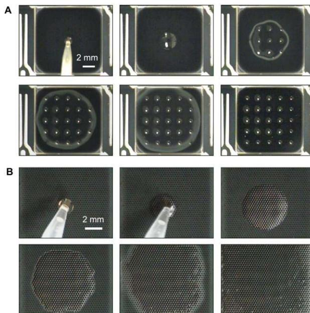
Fig. 7. Images showing (A) the spreading of 0.5  $\mu\text{L}$  of EMI-BF<sub>4</sub> on the CNT-coated surface of an emitter die with an array of 25 emitters in 1  $\text{cm}^2$  and (B) the spreading of 5  $\mu\text{L}$  of EMI-BF<sub>4</sub> on the CNT-coated surface of an emitter die with an array of 1900 emitters in 1  $\text{cm}^2$ .
