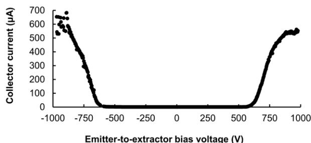
Fig. 9. Magnitude of the collector current as a function of the emitter-to-extractor bias voltage for an electro spray source with 1900 emitters in  $1 \text{ cm}^2$ .
