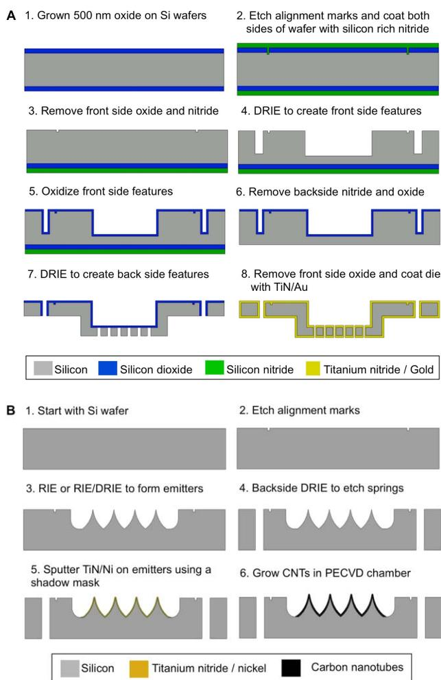
Fig. 2. (A) Process flow to fabricate the extractor grid dies; (B) process flow to fabricate the emitter dies.
