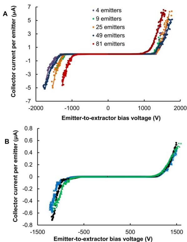
Fig. 10. Collector current per emitter as a function of emitter-to-extractor bias voltage for (A) the electrospay sources with 4, 9, 25, 49 and 81 emitters in  $1 \text{ cm}^2$  and (B) the electrospay sources with 1900 emitter in  $1 \text{ cm}^2$  showing the results of three different series of voltage sweeps.
