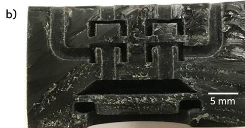
▲ Figure 1: (a) Design of the miniature diaphragm pump, and (b) image of a pump printed in one piece.
