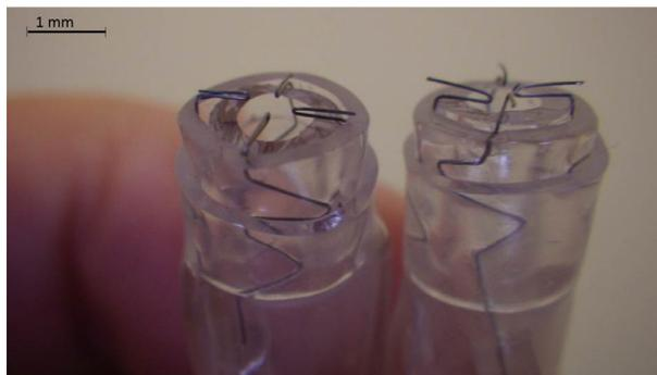
▲ Figure 1: A picture of two electrode assemblies. The target wire is installed at the center of the structure. The resulting plasma sputters metal atoms from the target, which then are carried towards the substrate by the gas flow and the electrostatic drag.
