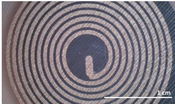
▲ Figure 1: Spiral printed using copper-doped thermoplastic.
