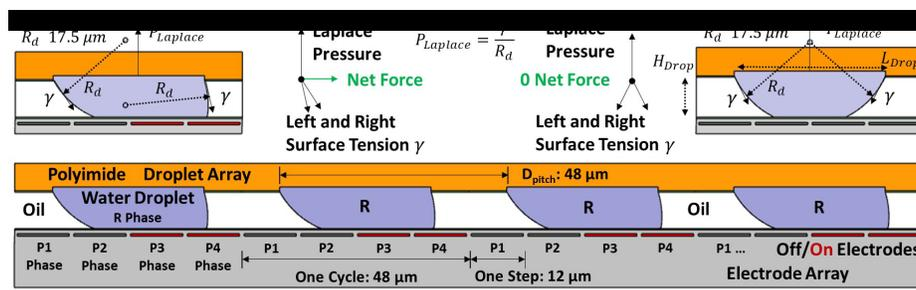
▲ Figure 1: Operating principle of microhydraulic actuators. Water droplets are shifted along by applying sequential electrical phases. From Kedzierski et al., *Science Robotics* 3, no. 22, eaat5643, 2018.
