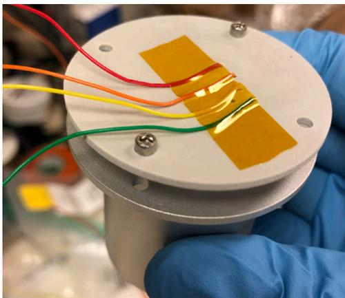
◀ Figure 2: A partially assembled retarding potential analyzer.
