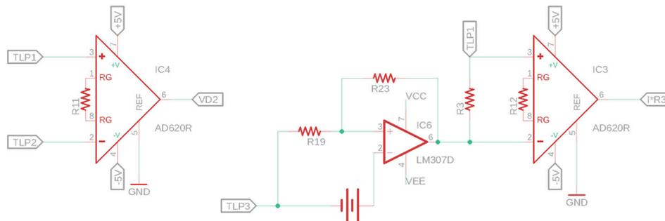
▲ Figure 1: Integrated circuit design for triple LP.
