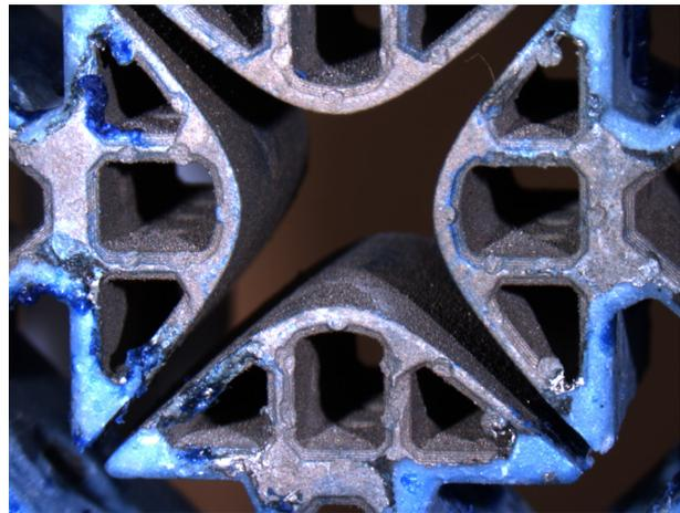
▲ Figure 2: Close-up photo of metallized, 3D-printed electrodes.
